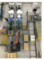
bags/hour and a 4-axis KUKA robotic arm. A special clamp that can receive both the empty pallet and the cardboard tray at the base of the pallet.
